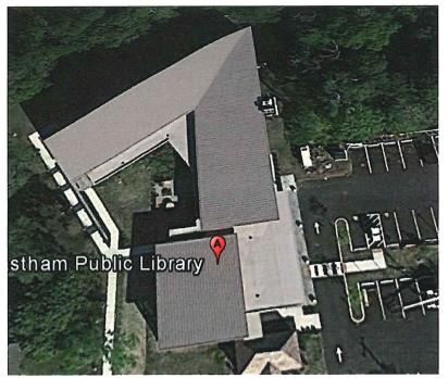
122' X 40' and 129' X 40' = 600 modules at 300 watts = 180,000 watts = 180kW = 237,780 kWh / year
